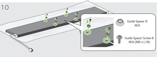
• Guide Spacer B (4ea) and Guide Spacer Screw B (4ea) are provided as accessories for wall-mounted OLW480B.
